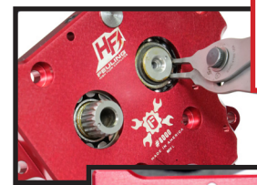
Verify the cams rotate freely & the timing marks are aligned.
