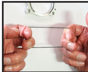
Lubricate O-rings and stretch O-rings if needed.
