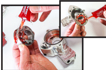
Lubricate the inner & outer gear sets.
