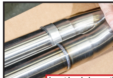
Insert head pipe section, do not tighten clamp
