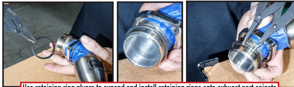
Use retaining ring plyers to expand and install retaining rings onto exhaust port spigots
