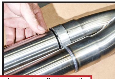
Loosely install head pipe clamp onto collector section
