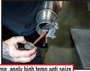
Install muffler to head pipe clamp, apply high temp anti seize
