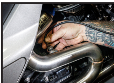
Use high heat anti seize on threads of each O2 sensor, thread into pipe
