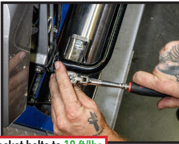
Final torque muffler bracket bolts to 18 ft/lbs
