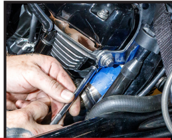
Slowly begin tightening down exhaust nuts, alternating between front & rear final torque to 120 in/lbs
