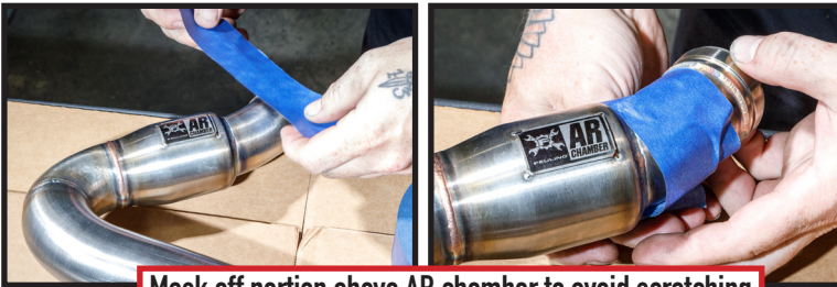
Mask off portion above AR chamber to avoid scratching
