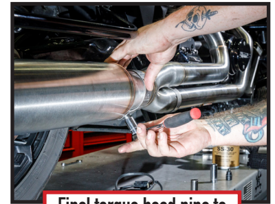
Final torque head pipe to muffler clamp to 22 ft/lbs.
