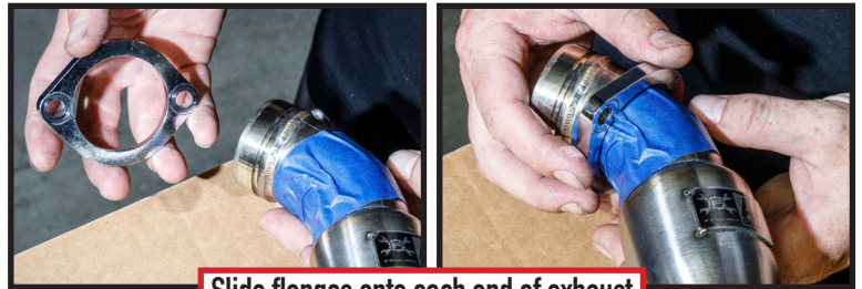
Slide flanges onto each end of exhaust
