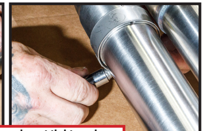
Insert head pipe section, do not tighten clamp
