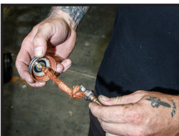
Use high heat anti seize on threads of each O2 sensor, thread into pipe
