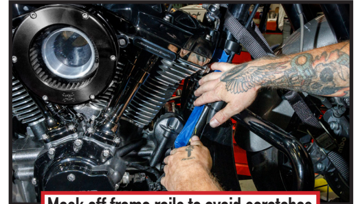
Mask off frame rails to avoid scratches
