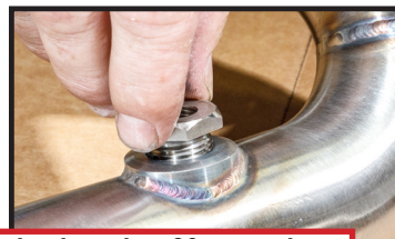
Apply high heat anti-seize, thread reducer into O2 sensor bung
