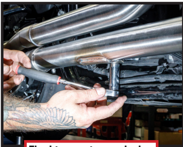
Final torque transmission bracket bolt to 20 ft/lbs.
