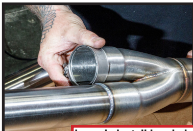
Loosely install head pipe clamp onto collector section
