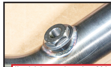
Hand tighten reducer into O2 bung, final torque reducer to 14 ft/lbs
