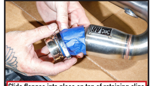
Slide flanges into place on top of retaining clips
