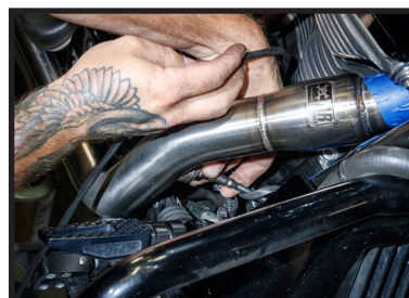
Final torque O2 sensors to 14 ft/lbs.
