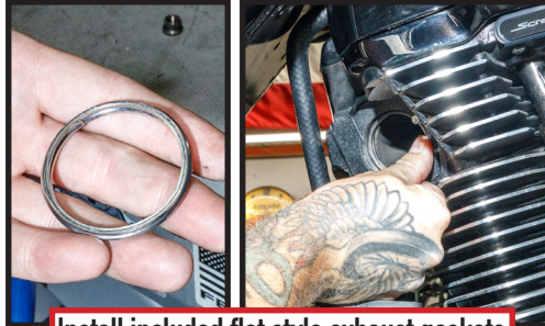
Install included flat style exhaust gaskets
