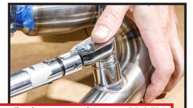
Hand tighten reducer into O2 bung, final torque reducer to 14 ft/lbs
