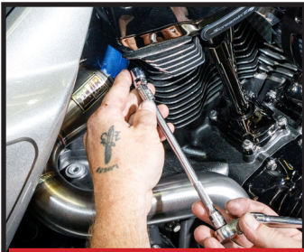
Slowly begin tightening down exhaust nuts, alternating between front & rear final torque to 120 in/lbs
