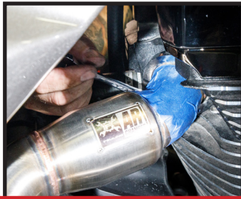
Slowly begin tightening down exhaust nuts, alternating between front & rear final torque to 120 in/lbs
