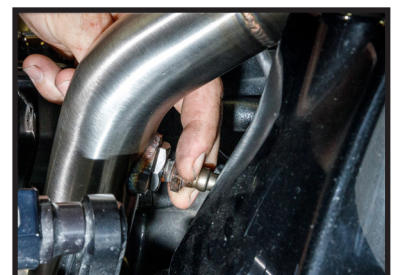
Final torque O2 sensors to 14 ft/lbs.
