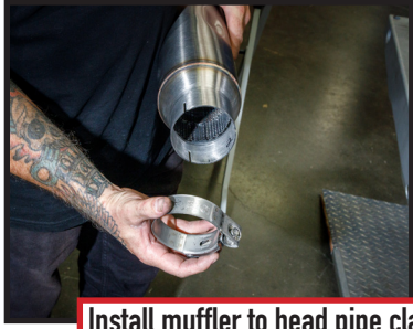
Install muffler to head pipe clamp, apply high temp anti seize
