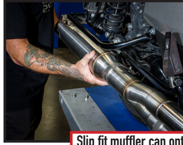
Slip fit muffler can onto head pipe until fully seated Loosely install Muffler bracket bolts
