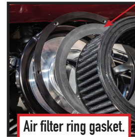
Line up metal rib with pillar on cage
