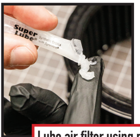
Lube air filter using provided O-ring lube
