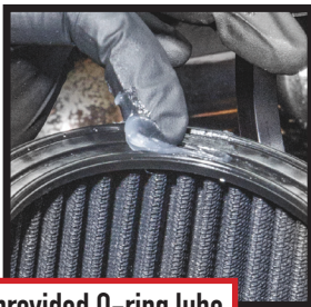
Lube air filter using provided O-ring lube
