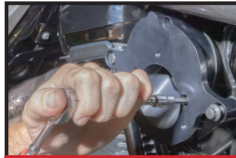
Torque throttle body bolts 72 in/lbs. Backing plate bolts to 22-24 ft/lbs
