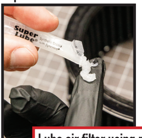
Lube air filter using provided O-ring lube
