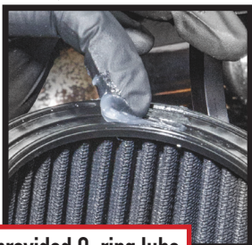
Lube air filter using provided O-ring lube
