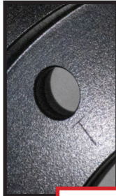
Clock T or S on air filter cage to top bolt hole.
