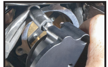
Locate breather hose. Apply thread sealant to barb fitting. Install tapered thread barb fitting snugly into backing plate. Install backing plate fitting
