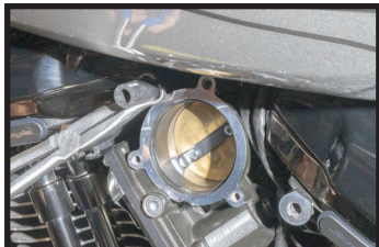
Locate breather hose. Apply thread sealant to barb fitting. Install tapered thread barb fitting snugly into backing plate. Install backing plate fitting
