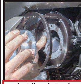
Install gasket and velocity stack inside cage
