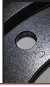
Clock T or S on air filter cage to top bolt hole.
