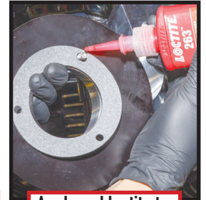
Apply red loctite to velocity stack bolts
