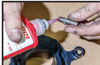
Locate breather hose. Apply thread sealant to barb fitting. Install tapered thread barb fitting snugly into backing plate. Install backing plate fitting
