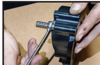
Locate breather hose. Apply thread sealant to barb fitting. Install tapered thread barb fitting snugly into backing plate. Install backing plate fitting
