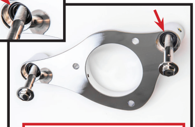
Install breather bolts with outer breather O-rings
