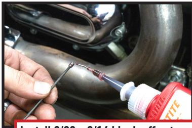
Install 8/32 x 3/16 block off set screw using 5/64 allen key (use 545 loctite)
