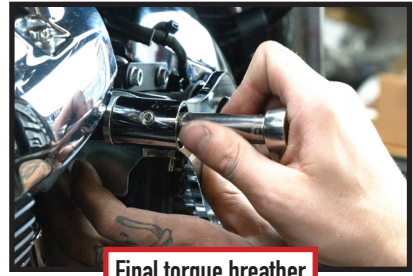
Final torque breather bolts to 22-24 ft/lbs.
