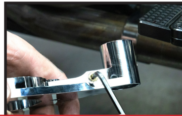
Remove bottom port 1/16 NPT plugs (both sides) using 5/32 allen key
