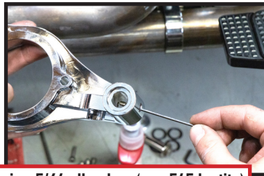
Install 8/32 x 3/16 block off set screw using 5/64 allen key (use 545 loctite)
