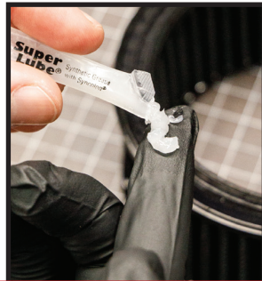
Install filter gasket ring into cage, Lube both filter bases with O-ring lube and install into cage
