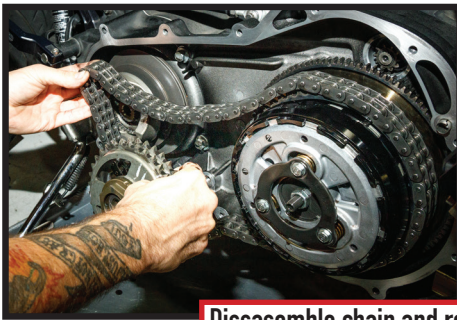
Dissassemble chain and remove compensator ramp
