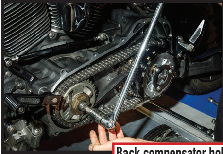
Back compensator bolt out one full turn
