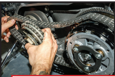
Re install sprocket and chain assembly, loosely thread compensator bolt into place
