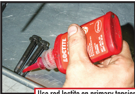
Use red loctite on primary tensioner bolts, final torque to 21-24 ft/lbs
