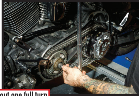
Back compensator bolt out one full turn
